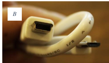
Figure 5: (A) Competition approved phone, (B) Micro to mini USB, (C) Micro port on PDM
